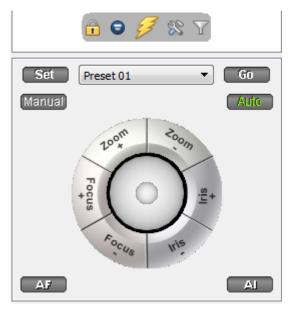
This panel provides controls for camera presets, and a software joystick for interactive control of the camera.
